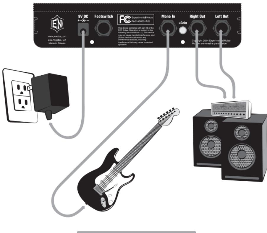
**Step 1:** Connect the instrument to the Mono In jack. If using a low signal level instrument, such as an electric guitar, press the +Gain switch so that it is in the in position.
