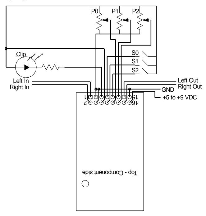
NOTES: Inputs and outputs have film capacitors on the module to block D.C. voltages.
